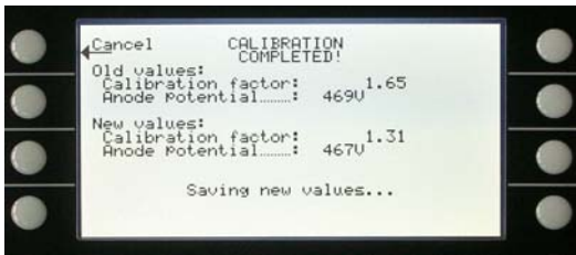
Fig. 39 Display: External Calibration, Step 7
