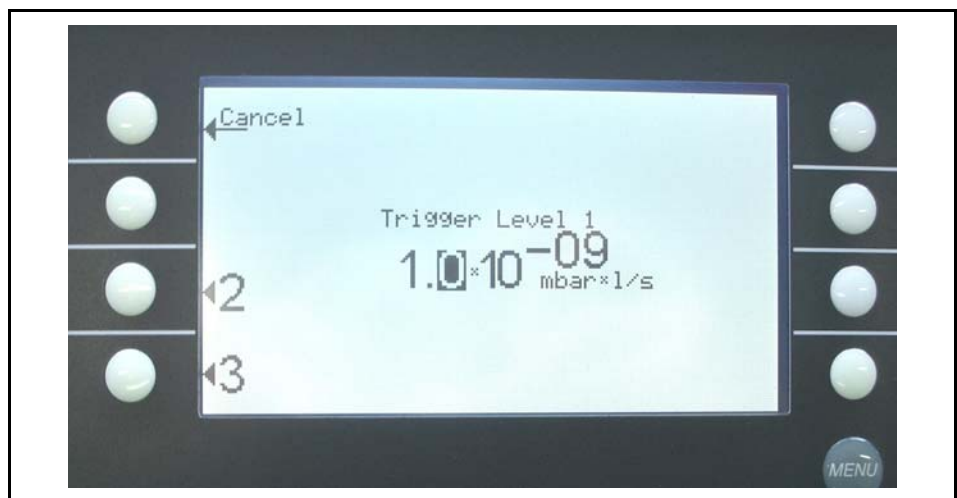
Fig. 16 Trigger level, change of the first digit
