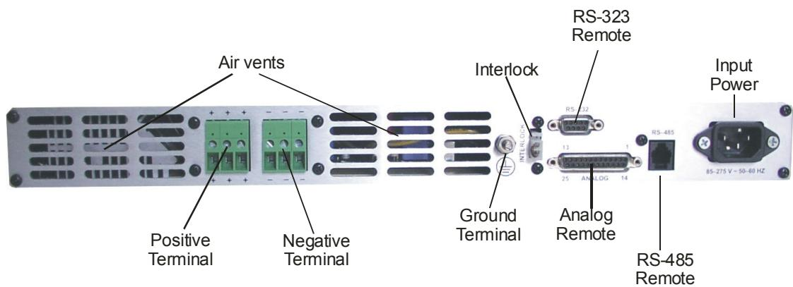
Fig 2-2 Emission Power Supply rear panel.
