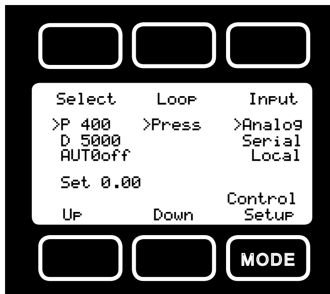
Figure 14. PC Series Control Setup Display
